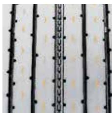
The S622 EFT is a premium free-rolling position trailer tire. The tread pattern features a decoupling groove to resist irregular wear and wide ribs to prevent damage caused by high-scrub applications. The S622 EFT is also a low-rolling resistance tire designed to maximize your mileage and fuel economy.
