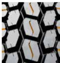
The S753 is an open shoulder drive, excellent for regional and pickup applications. Featuring a center interlocking tread block designed for improved stability, the S753 delivers exceptional tread life.
